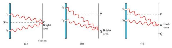
The distance L between the slits and the screen is typically large compared with the distance d between the slits, so that the light waves from the two slits to a point on the screen are essentially parallel. In this case, as can be seen from the construction below, the path difference between the two waves is given by
