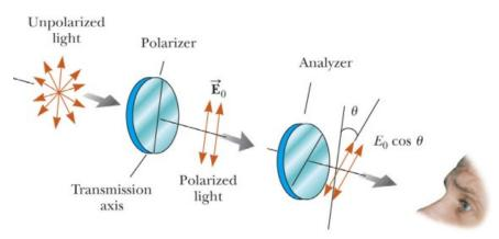
If  $E_0$  is the amplitude of the electric field of the polarized light before the analyzer, then the amplitude after the analyzer is  $E_0 cos \theta$ . Since the intensity of light is proportional to the square of the amplitude, then the final intensity is given by
