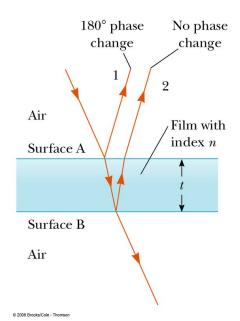
surface and no phase change will occur during the reflection from the bottom surface. For normal incidence, the path length difference between the two reflected waves is 2t, where t is the film thickness. A phase change of  $180^{\circ}$  is equivalent to the phase change that comes from a path length difference of one-half wavelength. Thus, in order for these two reflected waves to be in phase and interfere constructively, we must have
