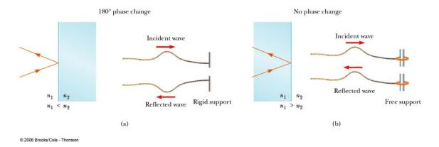
A similar situation occurs if a light rope and a heavy rope are tied together. There will be reflection at the junction of the ropes. If the wave travels from the light rope toward the heavy rope (fast to slow), then the reflected wave will be inverted. If it travels from the heavy rope to the light rope (slow to fast), then the reflected wave will not be inverted.
