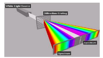
For a grating, the deviation of the diffracted light from its incoming direction increases with increasing wavelength, whereas for a prism it increases with decreasing wavelength.
