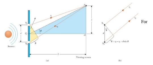
constructive interference (bright lines), the path difference must be an integral number of wavelengths. That is,
