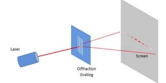
The path length difference between the waves from adjacent slits is an integral number of wavelengths. The conditions for the interference maxima (the bright spots) are the same as for a double slit, that is
