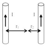
At the point in question, the field due to the left wire points into the page and the field due to the right wire points out of the page. Letting out of the page be the positive direction (this is arbitrary), we have
