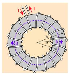
where  $L = 2 \pi r$ . The toroid is a useful device used in everything from tape heads to tokamaks (nuclear fusion reactor).
