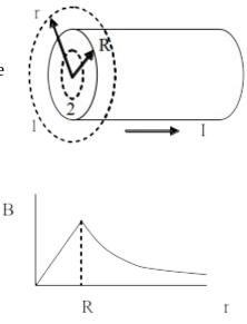
So, the magnetic field at the center of the wire is zero and it is a maximum on the surface of the wire.
