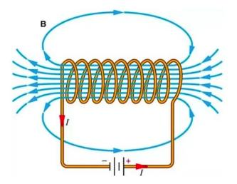
To calculate **B** inside, we pick a rectangular loop as shown to the right, part of which is inside and part of which is outside. The only contribution to the integral in Ampere's law is from the path 1. Paths 2 and 4 are perpendicular to **B** (dot product is zero) and outside the field is weak. If the loop has length l and encloses N turns, then we have
