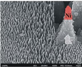
Electron Micrograph of an array of silicon nanopillars, the top of which was coated by electrodeposition with a magnetic material.
