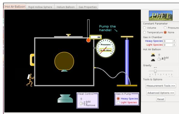
The sphere is like a hot air balloon. Its mass is not specified but assume it to be non-zero. Different molecules of air can enter and leave its volume and its temperature inside can be changed. Set *Gravity* to the second mark from the left (it might be already set this way).
