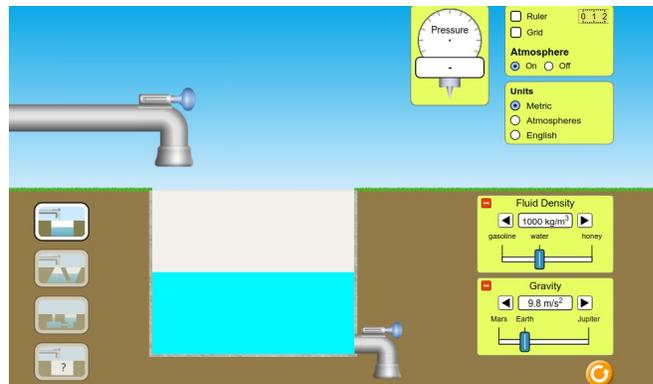
Select to display *Grid* and set *Atmosphere off*. You can drag around the pressure ‘clock’ to read the pressure at different locations and use the ruler to measure the depth. Fill up the tank with water using the tap.
