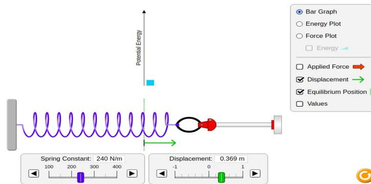
Select energy plot, values, displacement, applied force and equilibrium position and the spring constant to 300N/m.
