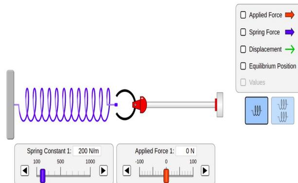
Set the spring constant 1 to be 100N/m and click the buttons to display the applied force, the spring force, the displacement and values.
