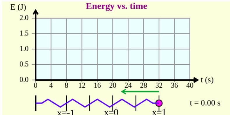
Set the spring constant to 2.0 N/m and mass of the ball 2.0 kg. Note the ball oscillates between -1m and 1m. Play the simulation:
