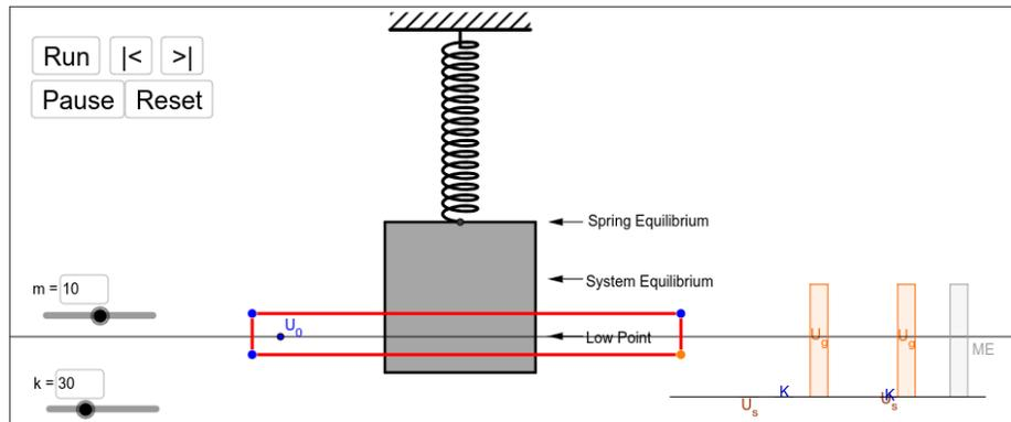
Select mass  $m = 10$  and spring constant  $k = 30$ . Three positions of the block are shown: they refer to the top side of the block. The columns on the right indicate the different forms of mechanical energy. Run the simulation and play close attention. The line labeled  $U_0$  is the reference height used to calculate the gravitational potential energy.
