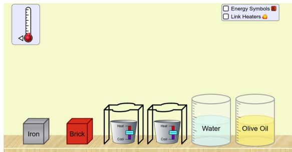
Here you will heat up a block and investigate how heat is exchanged with the liquid in a beaker. On the top left corner there is a thermometer. The marks range from  $25^{\circ}\text{C}$  to  $250^{\circ}\text{C}$ , the initial room temperature is just above  $25^{\circ}\text{C}$ . You can select and use as many thermometers as needed.
