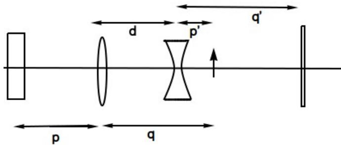
21. Measure  $p$  and use  $f$  of the converging lens and the equation (1) to calculate  $q$
