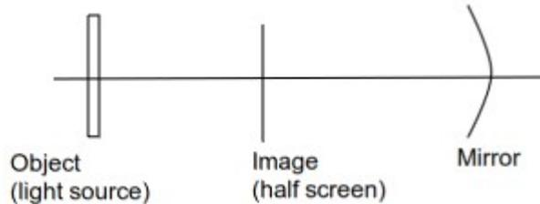
*Step 2.* Move the mirror and the half screen until the image is formed. Measure  $p$  and  $q$  and calculate the focal length.
