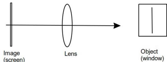
Step 2. Adjust the position of the lens on the bench such that the image (of the window for example) is formed on the screen.
