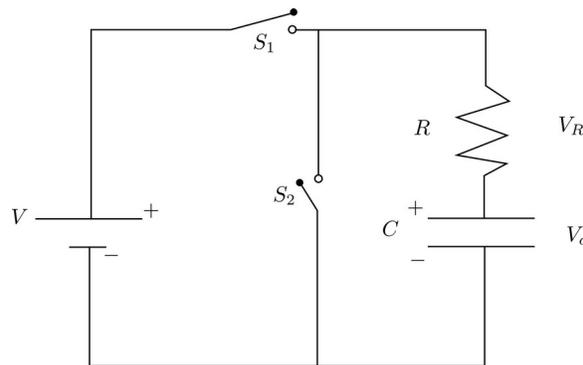
In the diagram above we display an RC circuit. When we close the switch  $S_1$  leaving the switch  $S_2$  open, the capacitor is **charged** through the resistor by the constant voltage source. The voltages across the capacitor and resistor change exponentially with time. The voltage across the capacitor and the resistor are given as,
